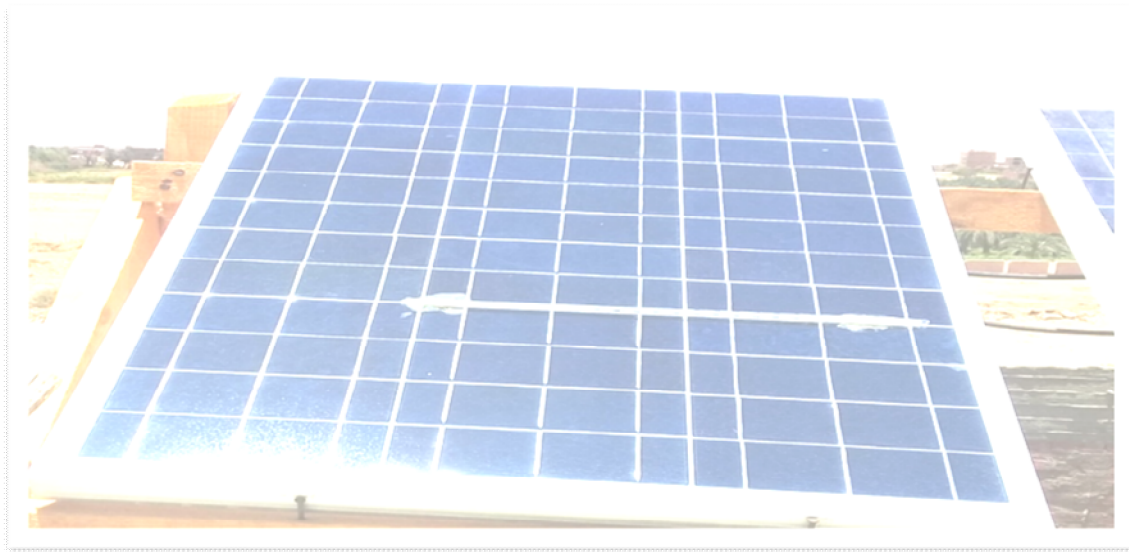
Figure 2. Photovoltaic (PV) panels with dimensions of 50.5 cm W X 69.5 cm L X 2.5 cm H, tilted at 30 degrees to ward south at El-Kharga to face the sun, with a thermometer of 0-100 °C scale.
